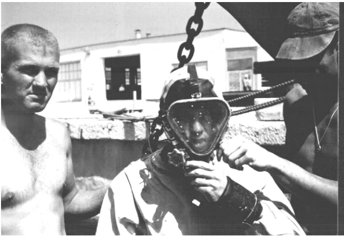
Student using Jack Brown shallow water diving apparatus. This rig was used aboard many Navy vessels for hull maintenance and screw clearing.
